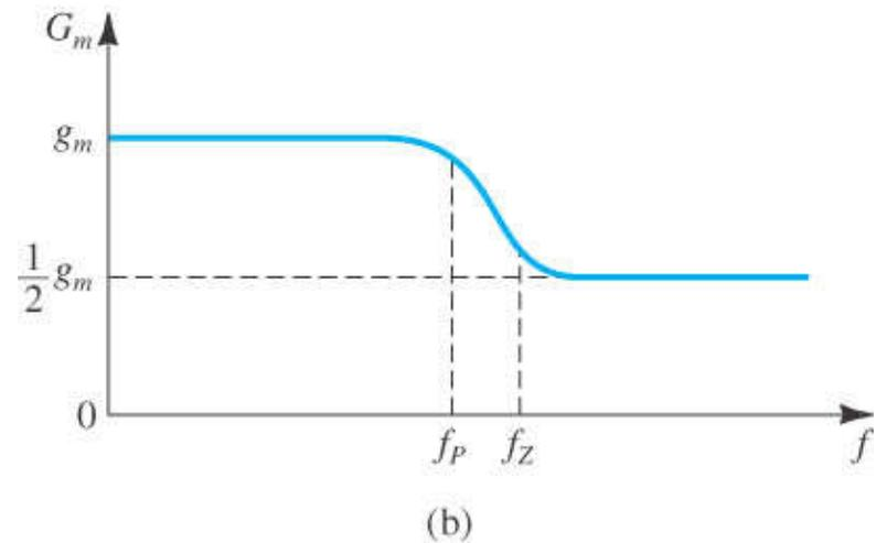
**Figure 7.39** (a) Frequency-response analysis of the active-loaded MOS differential amplifier. (b) The overall transconductance  $G_m$  as a function of frequency.
