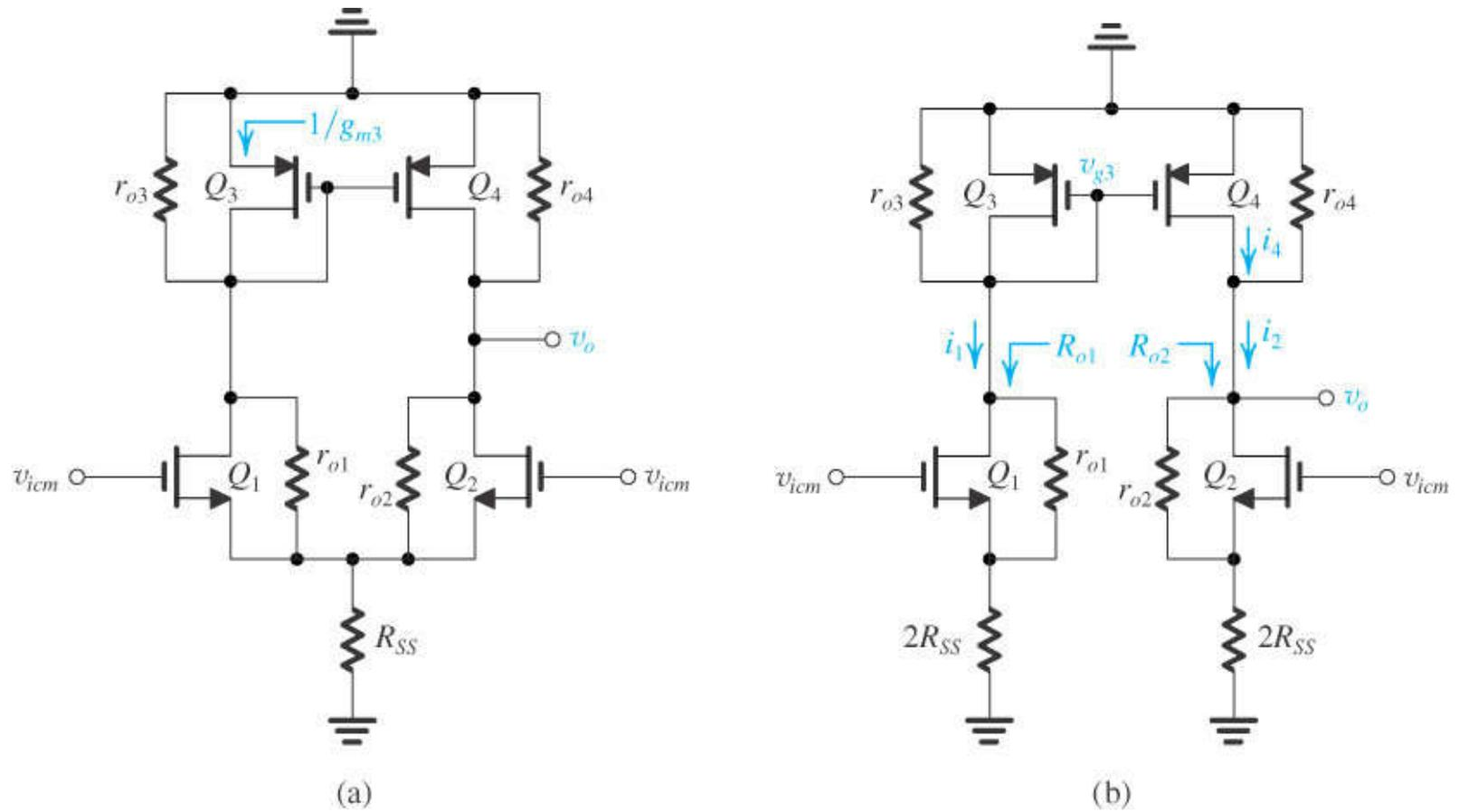
**Figure 7.31** Analysis of the active-loaded MOS differential amplifier to determine its common-mode gain.
