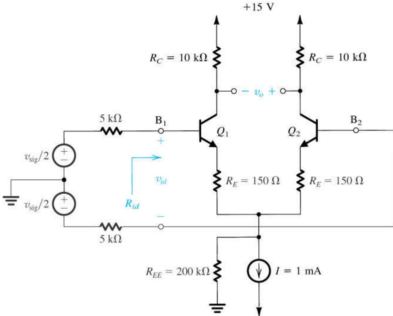
**Figure 7.24** Circuit for Example 7.1.
