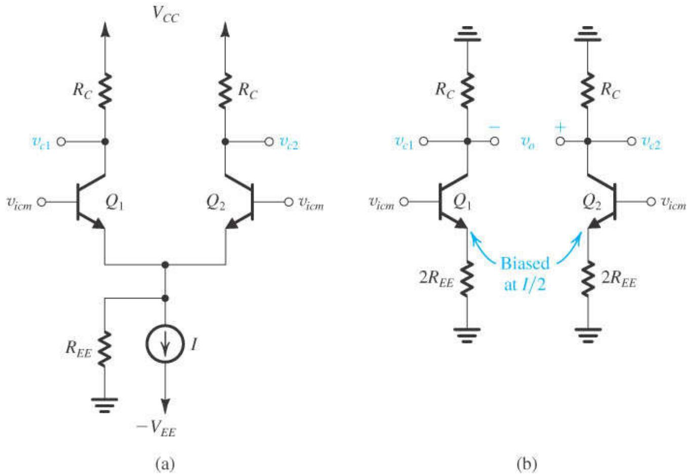
**Figure 7.22** (a) The differential amplifier fed by a common-mode voltage signal  $v_{icm}$ . (b) Equivalent “half-circuits” for common-mode calculations.
