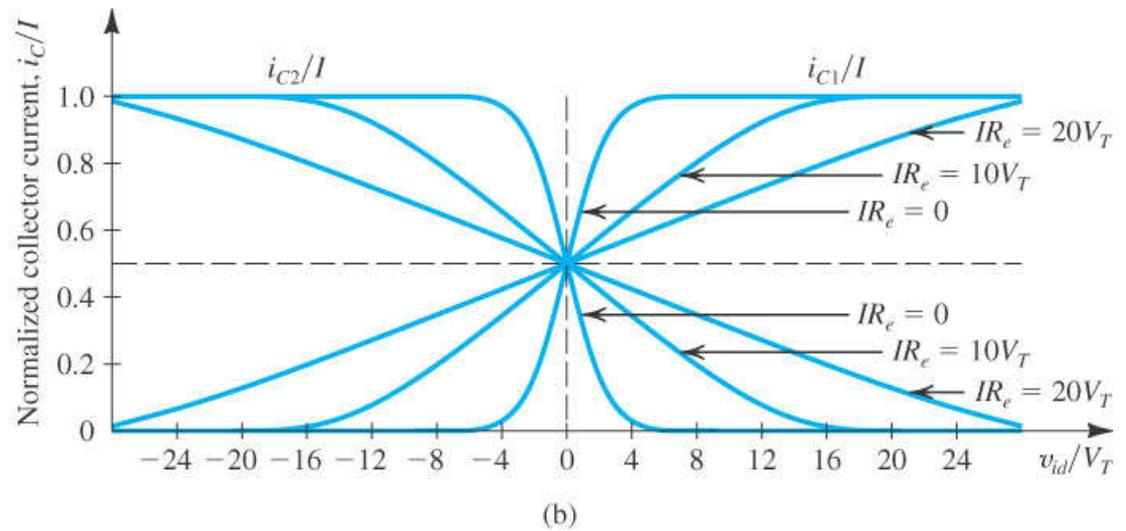
**Figure 7.15** The transfer characteristics of the BJT differential pair **(a)** can be linearized **(b)** (i.e., the linear range of operation can be extended) by including resistances in the emitters.
