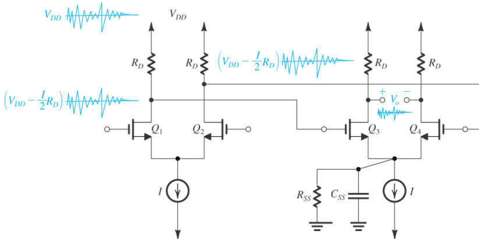
**Figure 7.38** The second stage in a differential amplifier is relied on to suppress high-frequency noise injected by the power supply of the first stage, and therefore must maintain a high CMRR at higher frequencies.
