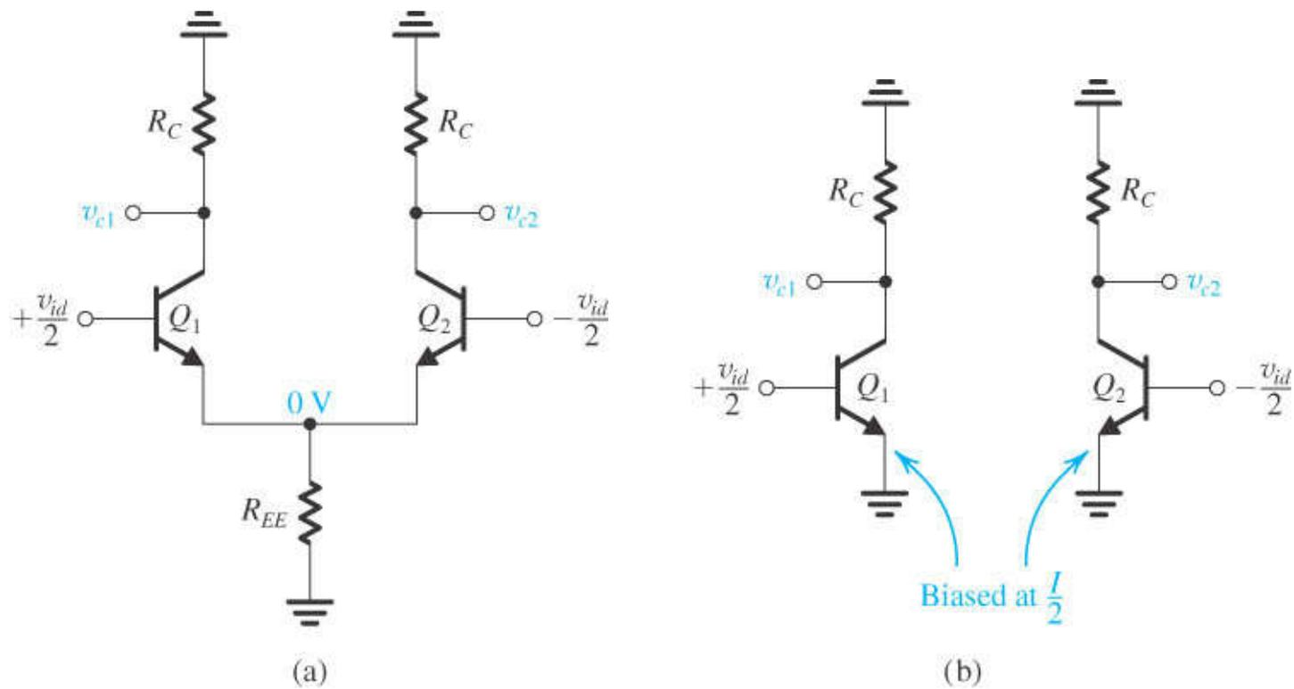
**Figure 7.19** Equivalence of the BJT differential amplifier in (a) to the two common-emitter amplifiers in (b). This equivalence applies only for differential input signals. Either of the two common-emitter amplifiers in (b) can be used to find the differential gain, differential input resistance, frequency response, and so on, of the differential amplifier.
