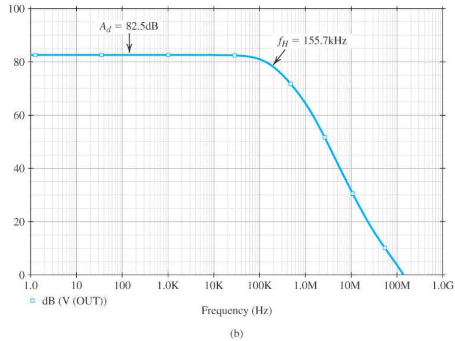
**Figure 7.53** Frequency response of (a) the op-amp circuit in Fig. 7.51 and (b) the op-amp circuit in Fig. 7.51 but with a resistor  $R'_3 = R_3$  inserted in the collector of  $Q_4$  to make the op-amp circuit symmetrical.
