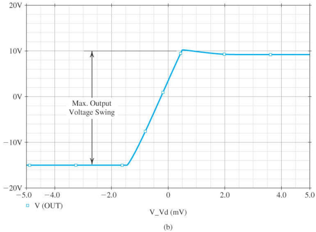
**Figure 7.52 (Continued) (b)** An expanded view of the transfer characteristic around the high-gain region.
