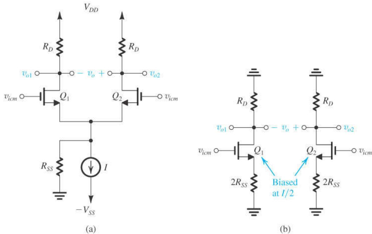
**Figure 7.10** (a) The MOS differential amplifier with a common-mode input signal  $v_{icm}$ . (b) Equivalent circuit for determining the common-mode gain (with  $r_o$  ignored). Each half of the circuit is known as the “common-mode half-circuit.”
