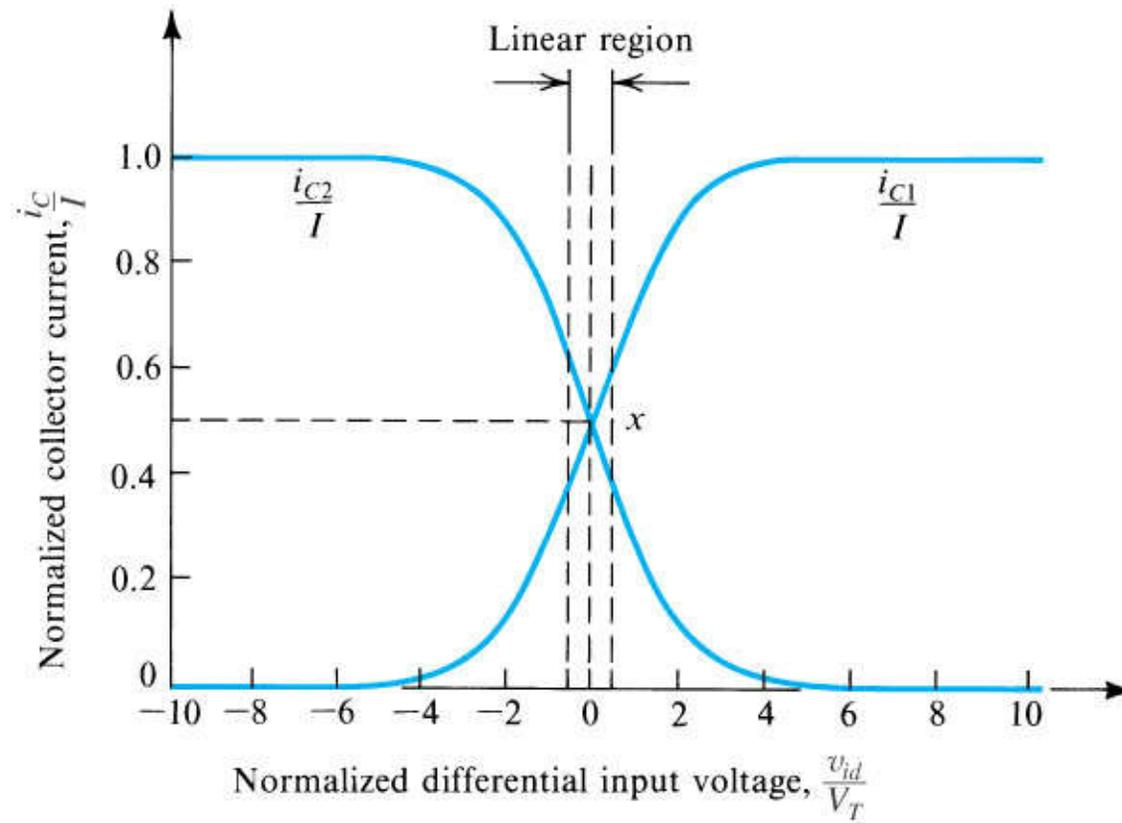
**Figure 7.14** Transfer characteristics of the BJT differential pair of Fig. 7.12 assuming  $\alpha = 1$ .
