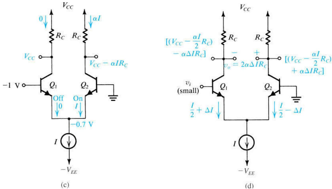
**Figure 7.13** (Continued) (c) The differential pair with a large differential input signal of polarity opposite to that in (b). (d) The differential pair with a small differential input signal  $v_i$ . Note that we have assumed the bias current source  $I$  to be ideal (i.e., it has an infinite output resistance) and thus  $I$  remains constant with the change in  $v_{CM}$ .
