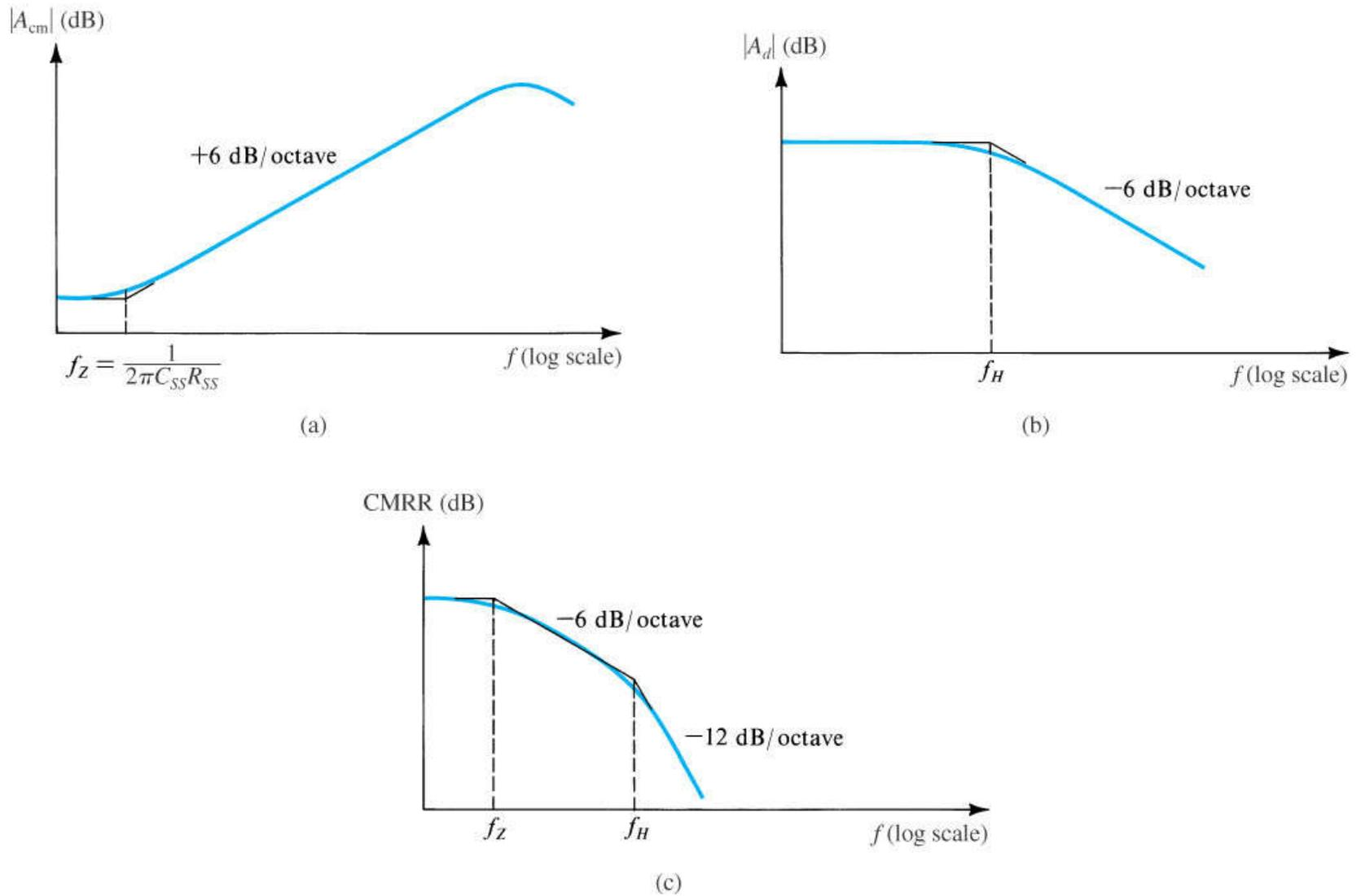
**Figure 7.37** Variation of (a) common-mode gain, (b) differential gain, and (c) common-mode rejection ratio with frequency.
