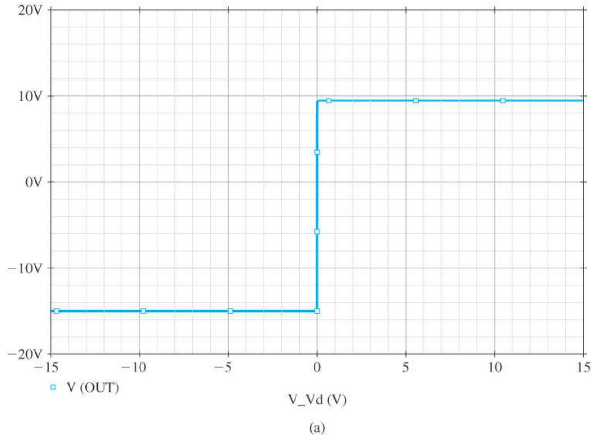
**Figure 7.52 (a)** The large-signal differential transfer characteristic of the op-amp circuit in Fig. 7.51. The common-mode input voltage  $V_{CM}$  is set to 0 V.
