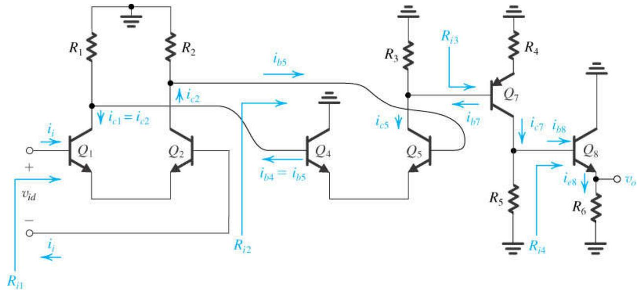
**Figure 7.49** The circuit of the multistage amplifier of Fig. 7.43 prepared for small-signal analysis. Indicated are the signal currents throughout the amplifier and the input resistances of the four stages.
