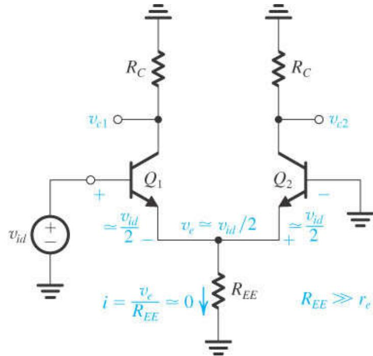
**Figure 7.20** The differential amplifier fed in a single-ended fashion.
