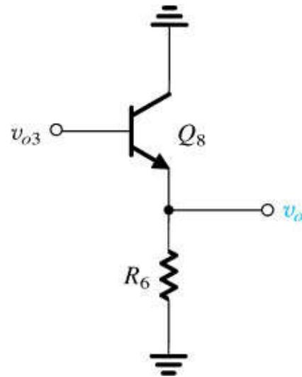
**Figure 7.48** Equivalent circuit of the output stage of the amplifier circuit of Fig. 7.43.
