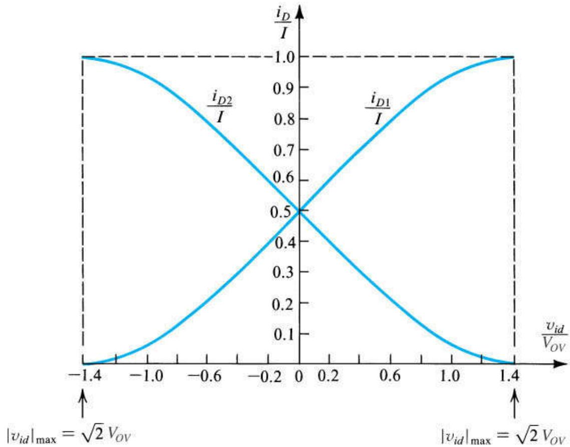
**Figure 7.6** Normalized plots of the currents in a MOSFET differential pair. Note that  $V_{OV}$  is the overdrive voltage at which  $Q_1$  and  $Q_2$  operate when conducting drain currents equal to  $I/2$ .
