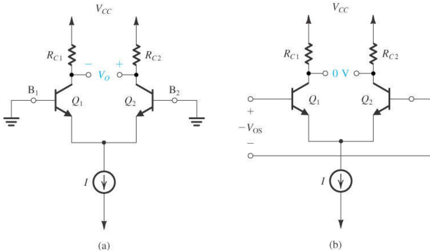
**Figure 7.26** (a) The BJT differential pair with both inputs grounded. Device mismatches result in a finite dc output  $V_O$ . (b) Application of the input offset voltage  $V_{OS}$ ;  $V_O/A_d$  to the input terminals with opposite polarity reduces  $V_O$  to zero.
