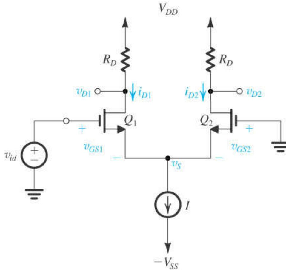
**Figure 7.4** The MOS differential pair with a differential input signal  $v_{id}$  applied. With  $v_{id}$  positive:  $v_{GS1} > v_{GS2}$ ,  $i_{D1} > i_{D2}$ , and  $v_{D1} < v_{D2}$ ; thus  $(v_{D2} - v_{D1})$  will be positive. With  $v_{id}$  negative:  $v_{GS1} < v_{GS2}$ ,  $i_{D1} < i_{D2}$ , and  $v_{D1} > v_{D2}$ ; thus  $(v_{D2} - v_{D1})$  will be negative.
