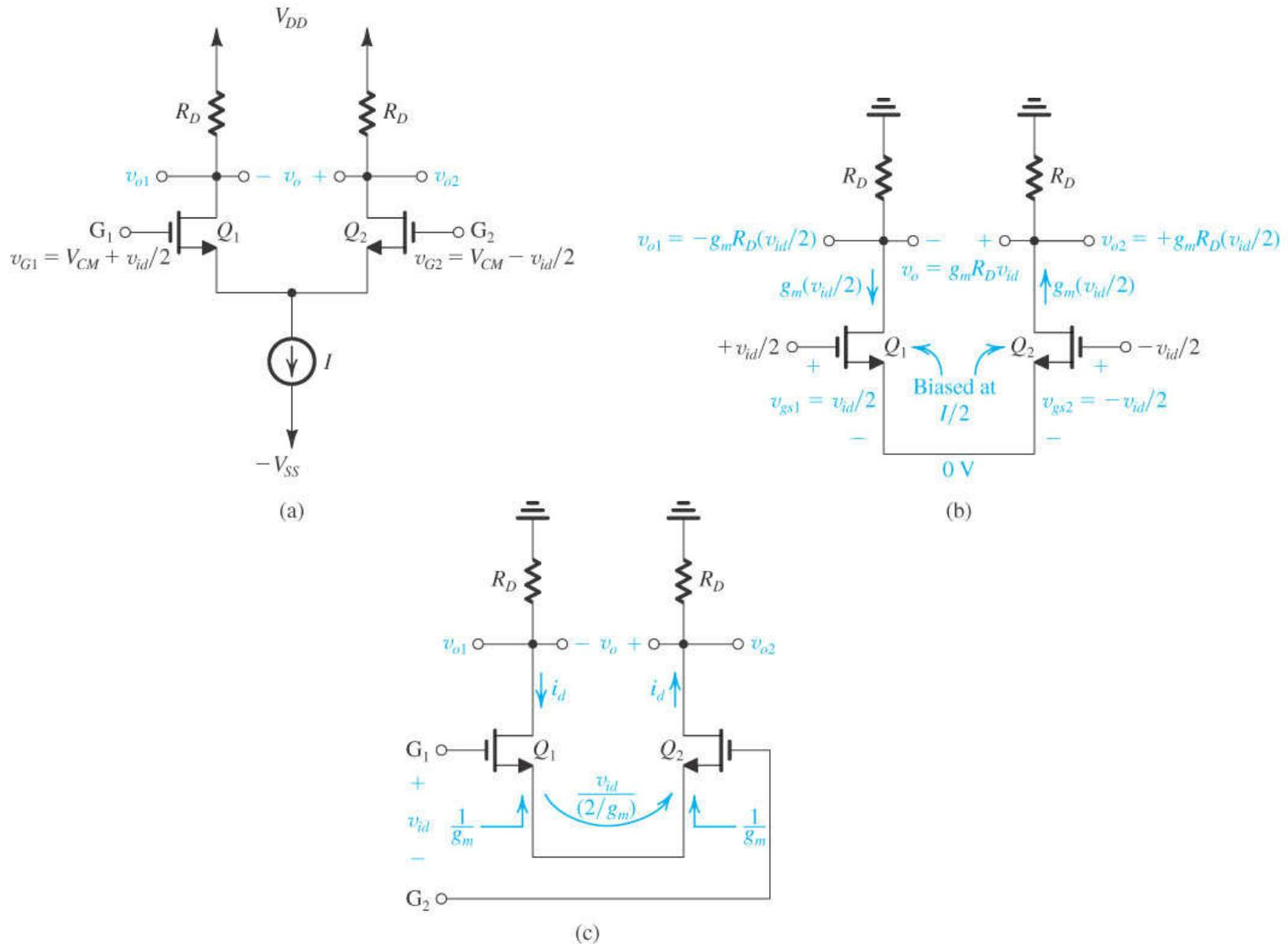
**Figure 7.8** Small-signal analysis of the MOS differential amplifier: (a) The circuit with a common-mode voltage applied to set the dc bias voltage at the gates and with  $v_{id}$  applied in a complementary (or balanced) manner. (b) The circuit prepared for small-signal analysis. (c) An alternative way of looking at the small-signal operation of the circuit.
