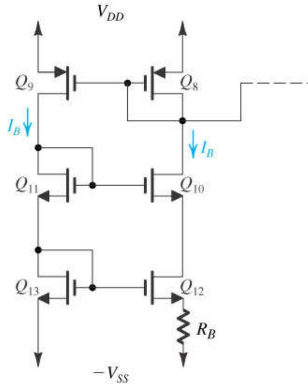
**Figure 7.42** Bias circuit for the CMOS op amp.
