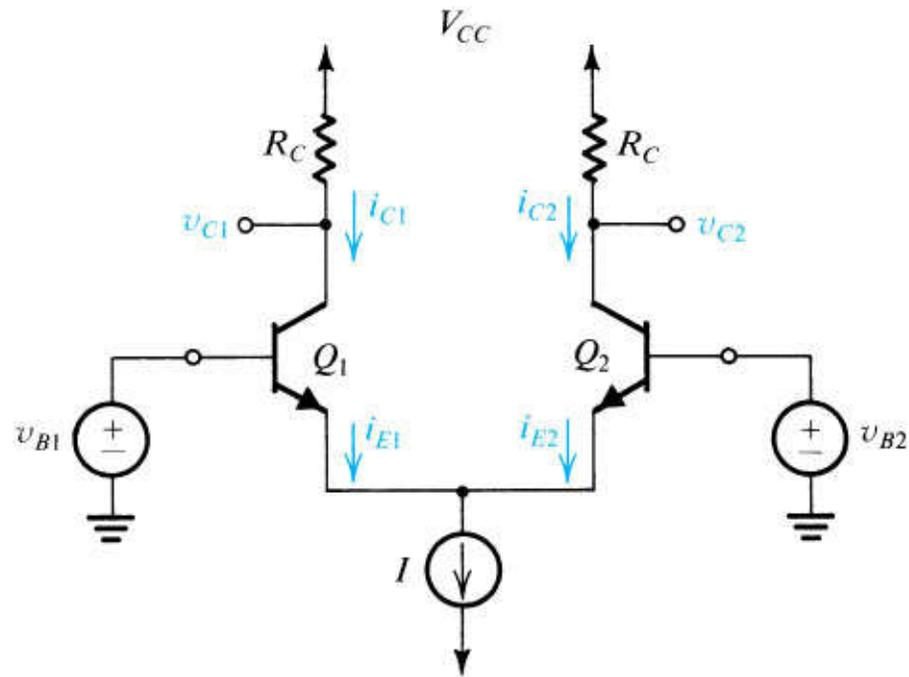
**Figure 7.12** The basic BJT differential-pair configuration.
