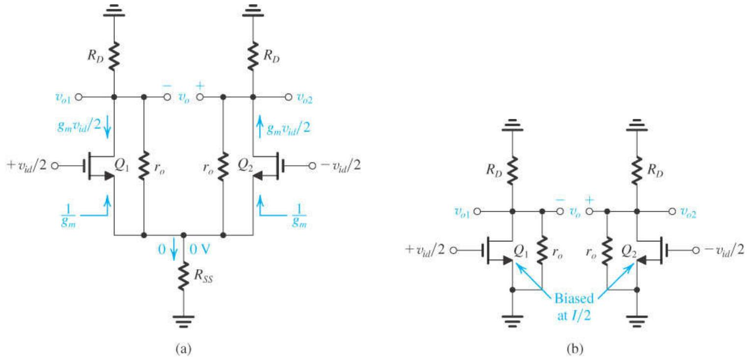
**Figure 7.9** (a) MOS differential amplifier with  $r_o$  and  $R_{SS}$  taken into account. (b) Equivalent circuit for determining the differential gain. Each of the two halves of the differential amplifier circuit is a common-source amplifier, known as its differential “half-circuit.”
