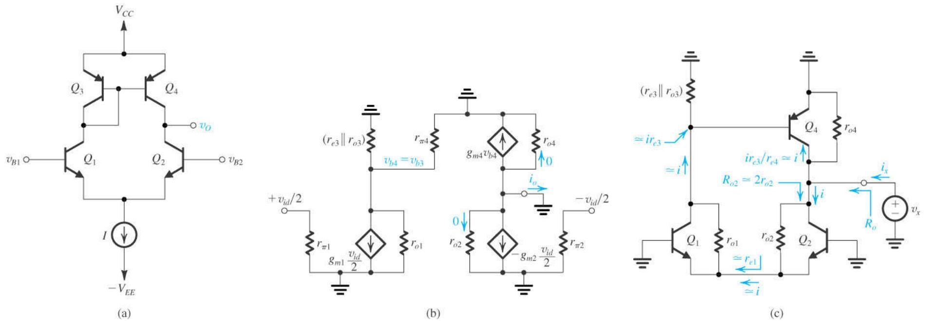
**Figure 7.32** (a) Active-loaded bipolar differential pair. (b) Small-signal equivalent circuit for determining the transconductance  $G_m$ ;  $i_o/v_{id}$ . (c) Equivalent circuit for determining the output resistance  $R_o$ ;  $v_x/i_x$ .
