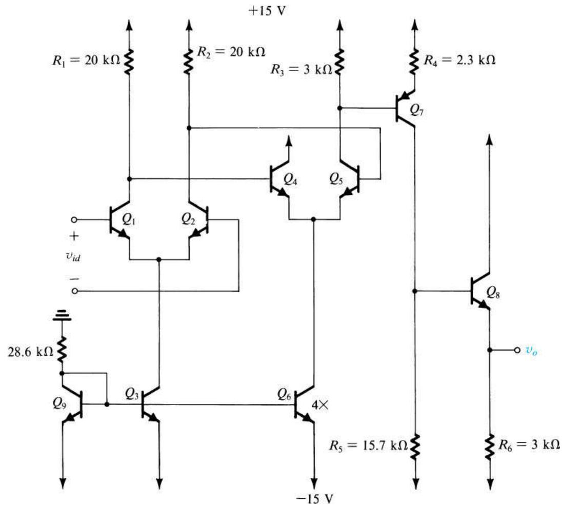
**Figure 7.43** A four-stage bipolar op amp.
