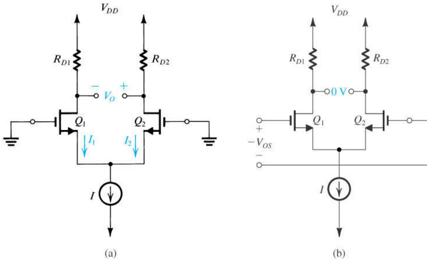
**Figure 7.25** (a) The MOS differential pair with both inputs grounded. Owing to device and resistor mismatches, a finite dc output voltage  $V_O$  results. (b) Application of a voltage equal to the input offset voltage  $V_{OS}$  to the terminals with opposite polarity reduces  $V_O$  to zero.
