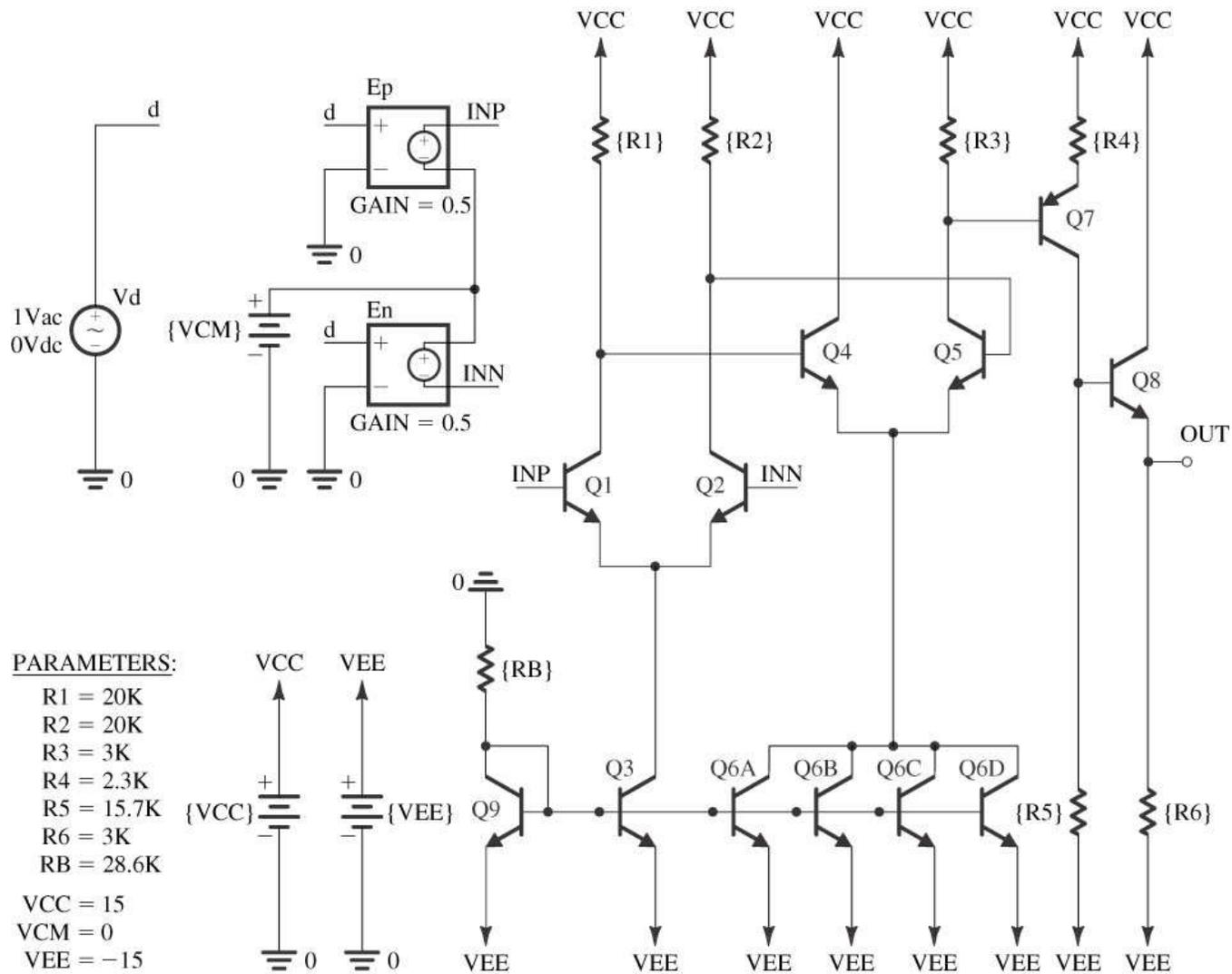
**Figure 7.51** Capture schematic of the op-amp circuit in Fig. 7.51.
