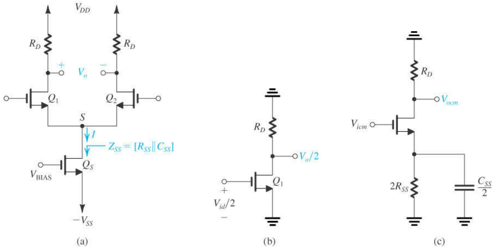
**Figure 7.36** (a) A resistively loaded MOS differential pair with the transistor supplying the bias current explicitly shown. It is assumed that the total impedance between node  $S$  and ground,  $Z_{SS}$ , consists of a resistance  $R_{SS}$  in parallel with a capacitance  $C_{SS}$ . (b) Differential half-circuit. (c) Common-mode half-circuit.
