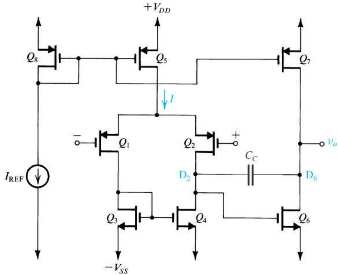
**Figure 7.40** Two-stage CMOS op-amp configuration.
