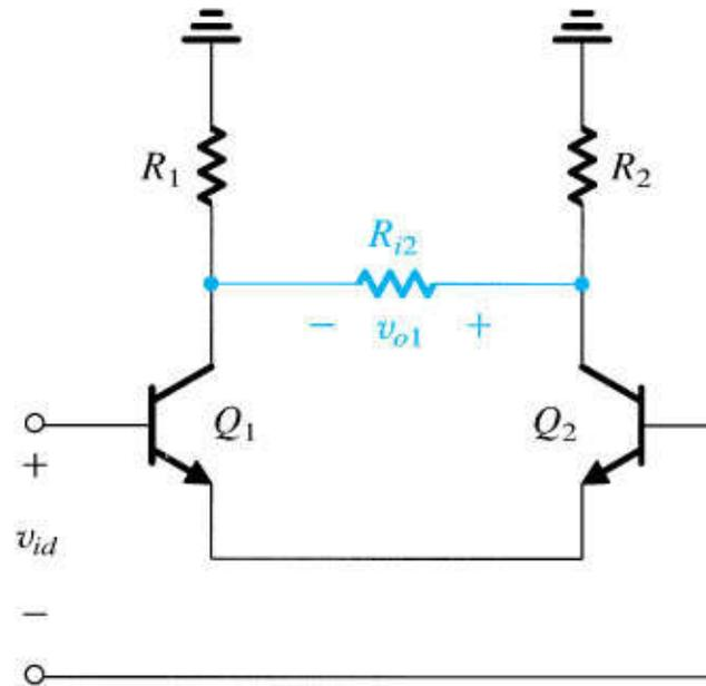
**Figure 7.45** Equivalent circuit for calculating the gain of the input stage of the amplifier in Fig. 7.43.
