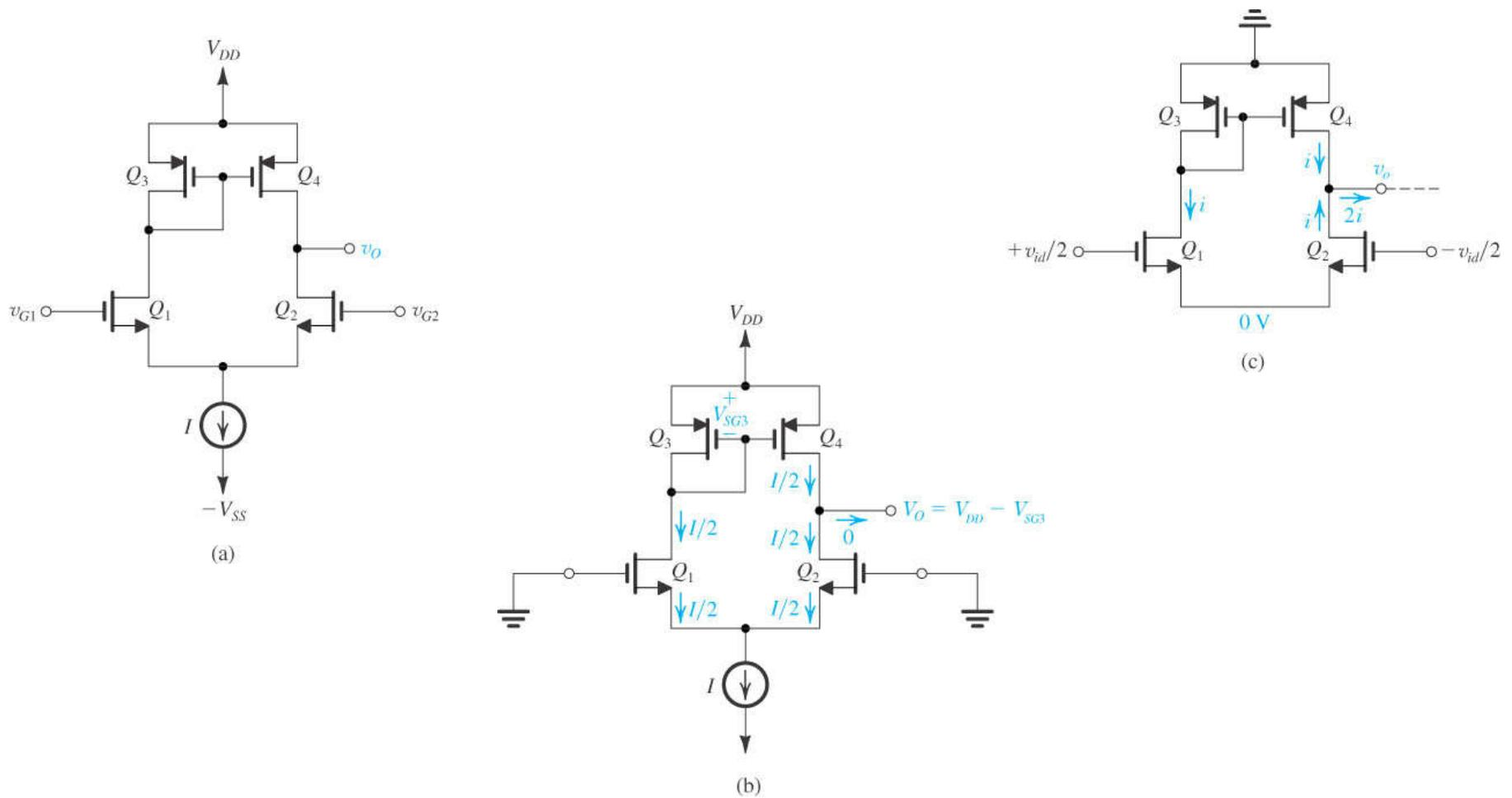
**Figure 7.28** (a) The active-loaded MOS differential pair. (b) The circuit at equilibrium assuming perfect matching. (c) The circuit with a differential input signal applied, neglecting the  $r_o$  of all transistors.
