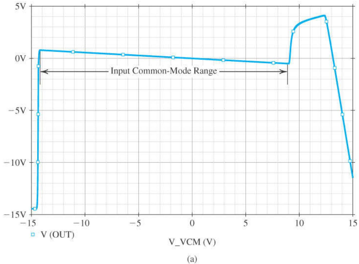
**Figure 7.54 (a)** The large-signal common-mode transfer characteristic of the op-amp circuit in Fig. 7.51. The differential input voltage  $v_d$  is set to  $-V_{\text{OS}} = -260.4 \mu\text{V}$  to prevent premature saturation.
