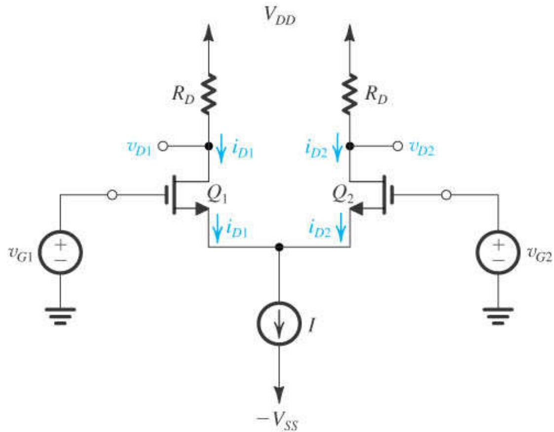
**Figure 7.1** The basic MOS differential-pair configuration.
