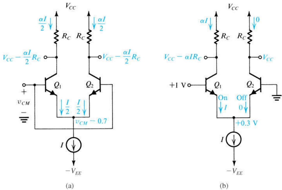
**Figure 7.13** Different modes of operation of the BJT differential pair: **(a)** The differential pair with a common-mode input signal  $v_{CM}$ . **(b)** The differential pair with a “large” differential input signal.
